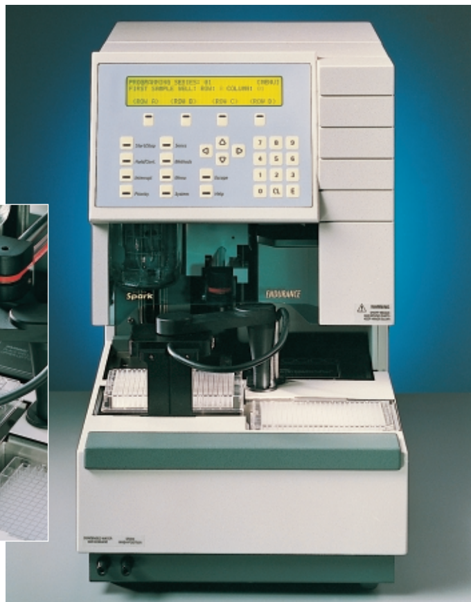
Well plate with x, y, z movement of the rack carriage.
