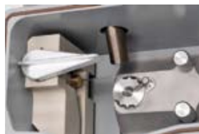
Detail of MSQ Plus with atmospheric pressure chemical ionization (APCI) installed
