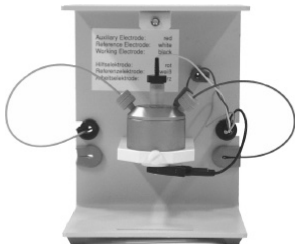
figure 5: electrochemical measurement cell EC4000, model Sputnik®
