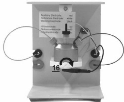
figure 14: measurement cell installed in the mounting device of the cell housing
