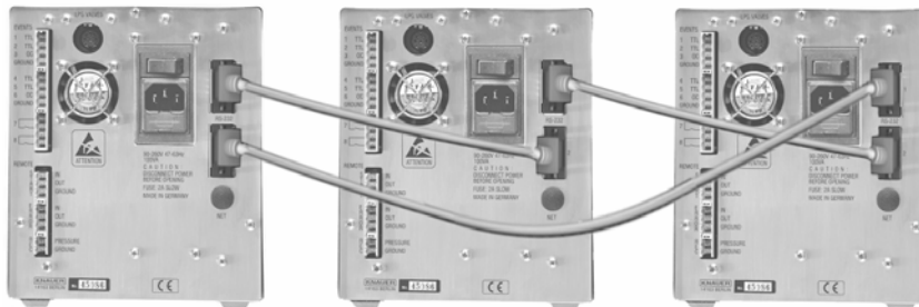
Fig. 23 Network of three instruments
