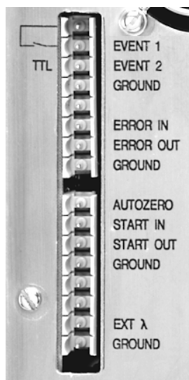
Fig. 22 Event and remote socket connections
