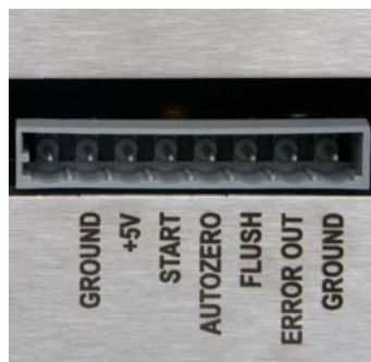
Fig. 15 Remote Control Connections
